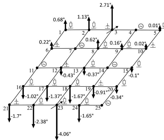
**Figure 11** Change of nodal voltage angles with angle control
