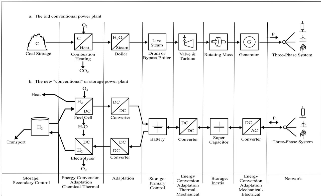
**Figure 1** Comparison between the existing fossil fuel based power plant (a) and the new storage power plant (b)
