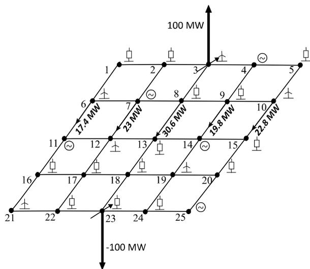
**Figure 8** Power flow with frequency control (not to scale)
