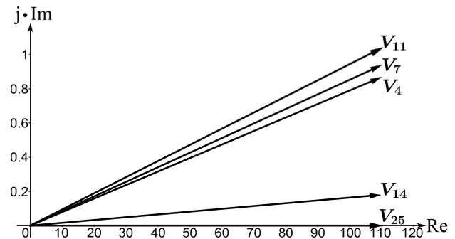
Figure 3 Voltage phasors of slacks (start of load flow)
