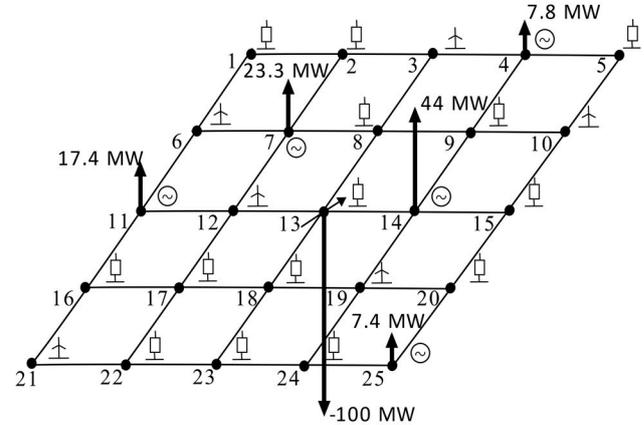
**Figure 6** Increase in power consumption in node 13 and the resulting increases in the generation of every slack
