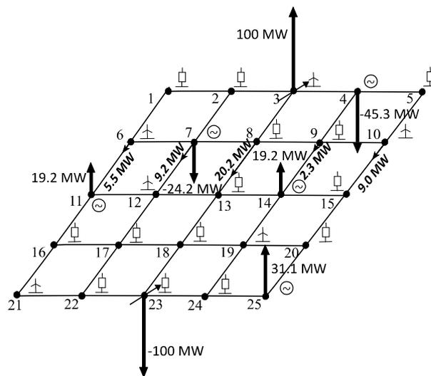
**Figure 10** Power flow with nodal voltage angle control (not to scale)
