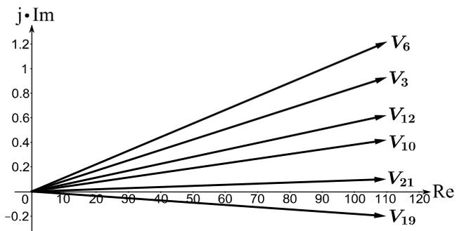
Figure 4 Voltage phasors of PV generators (start of load flow)
