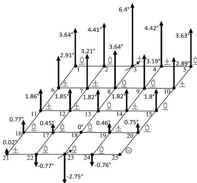
**Figure 9** Change of nodal voltage angles with frequency control
