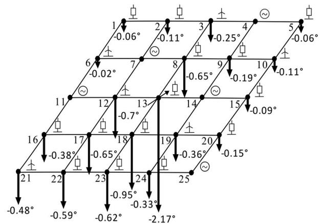
**Figure 7** Increase in power consumption in node 13 and the resulting angle changes in PV Generators and PQ consumers
