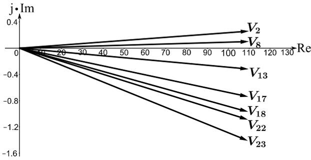
**Figure 5** Voltage phasors of selected PQ loads (start of load flow)
