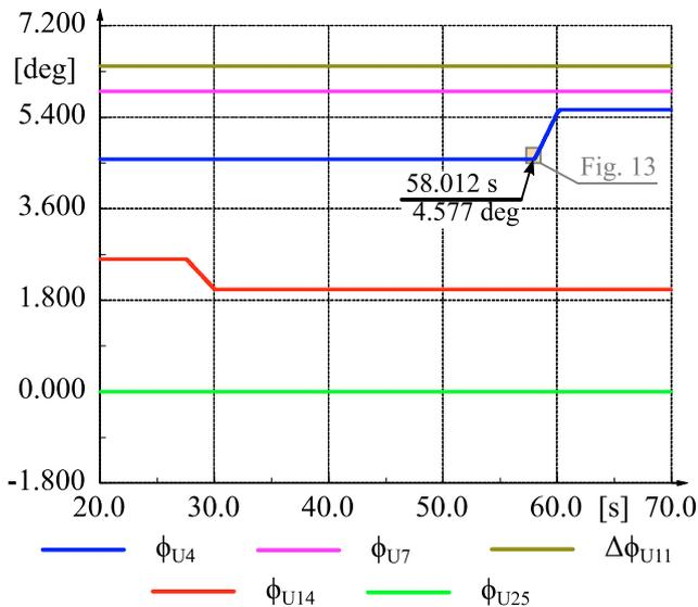
Fig. 12. Voltage angles of SPPs during wind ramp
