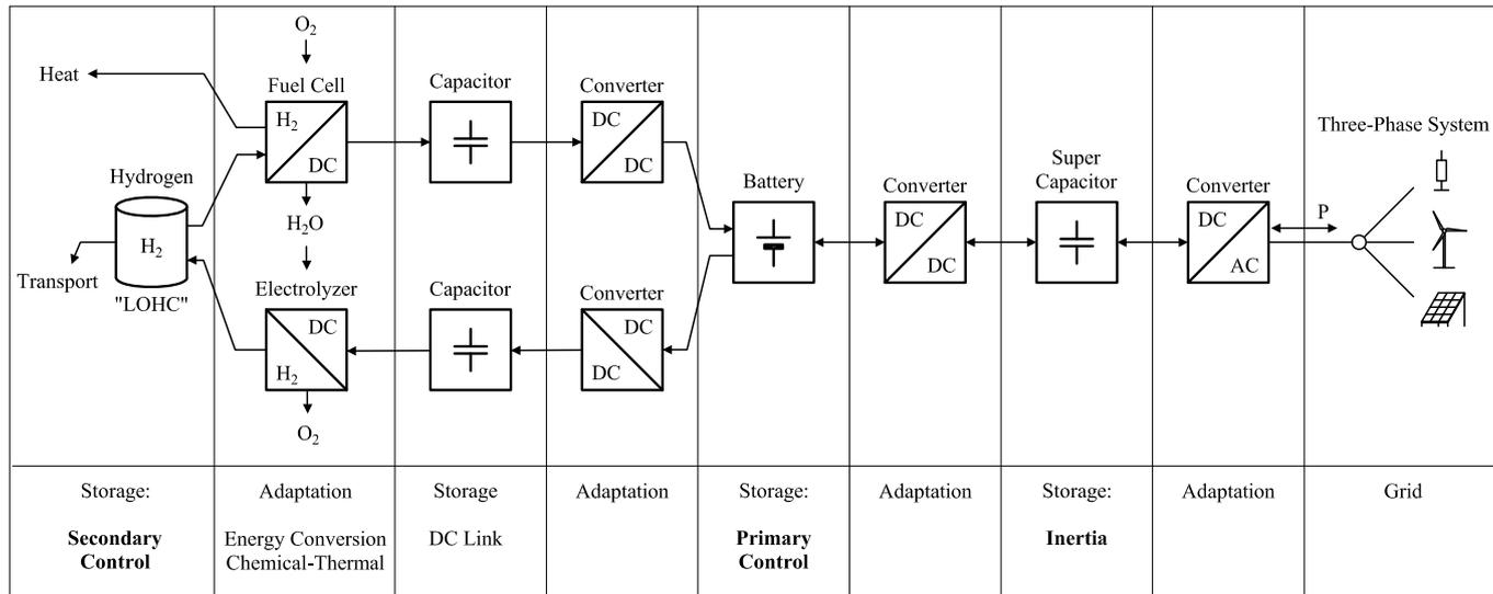
Fig. 2. Working principle of the internal components of a storage power plant (SPP)
