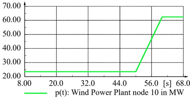
Fig. 9. Ramp increase in wind power at node 10
