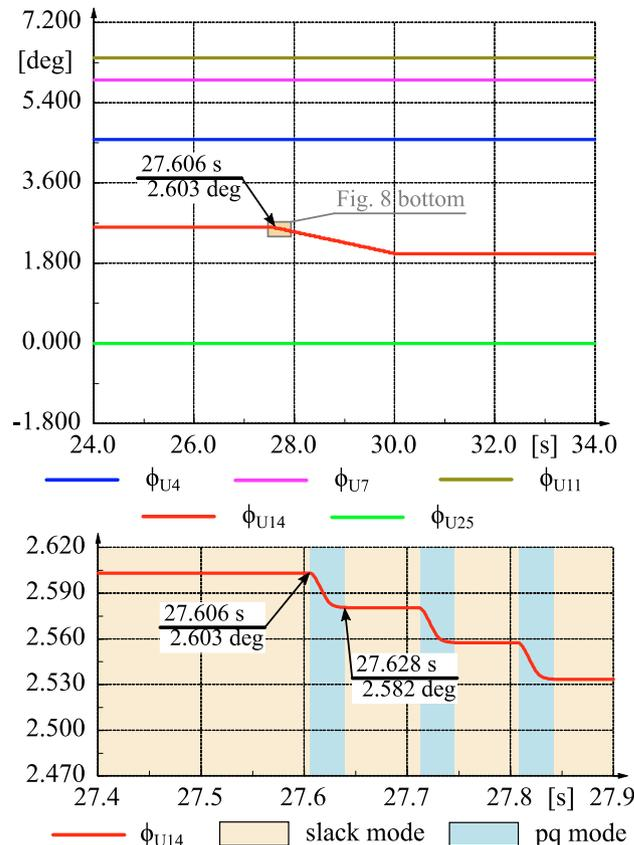
Fig. 8. Voltage angles of the SPPs during load ramp (top) and that of the SPP at node 14 upon reaching its maximum power limit (bottom)
