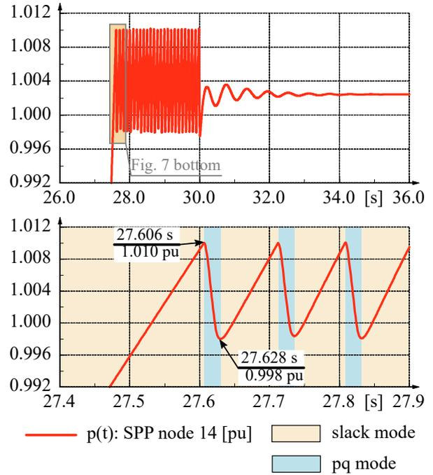
Fig. 7. Behaviour of SPP at node 14 upon reaching its maximum power limit
